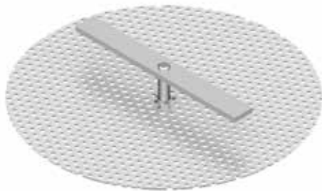
Fixed (secondary) strainer
